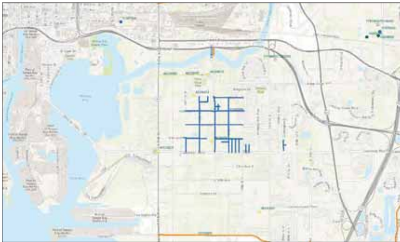
Figure 17-1B. Palm River Utilities service area to be converted to central sewer service.
