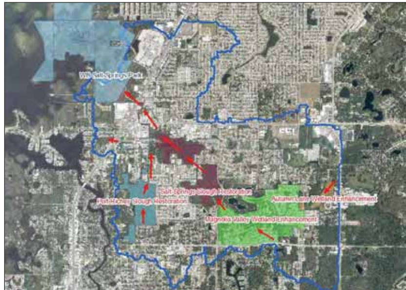
Figure 15-1C. Schematic of wetland enhancement and slough restoration areas in the Port Richey watershed.
