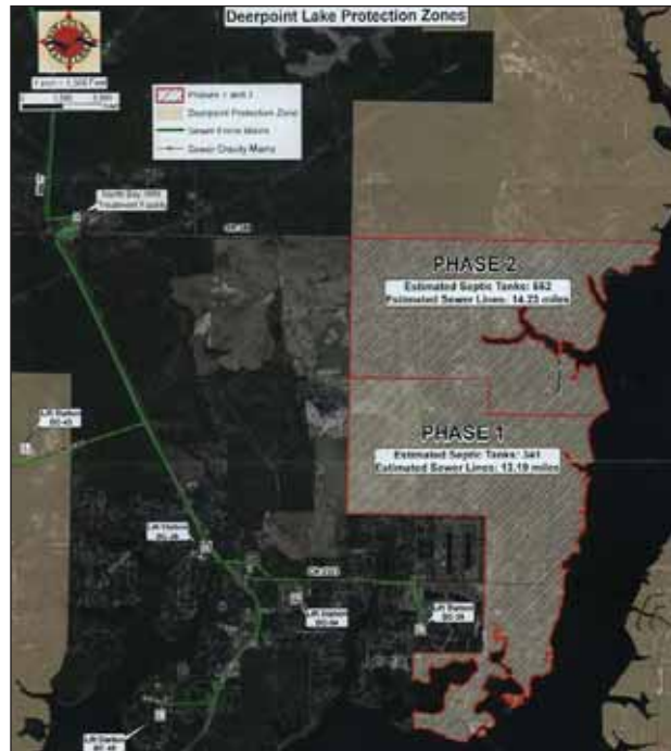
Figure 5-1C. Deer Point Lake area to be served by new centralized sewer facilities.
